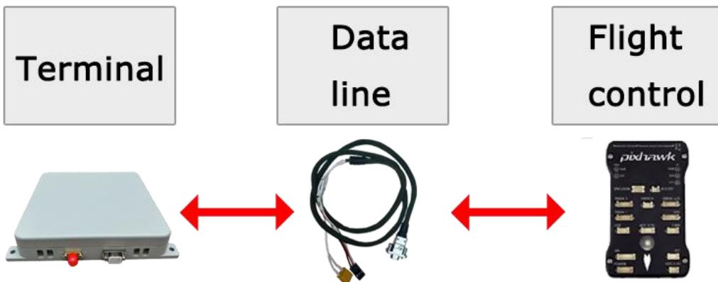
3. In RF signal access mode, this product replaces the conventional active antenna. When connecting using the RF interface of this product, please ensure that the interface of the connected party does not provide an over 5V power supply to this product to avoid possible power conflicts or damage. As shown in the following diagram.
